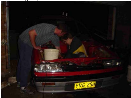
I hate this car! Al the drinks left so it was Luke and I working on the car at night. This is when we found out that the Silvia cross member doesn't bolt into o the front t of the car. So we left it with the s13 front cross member and front suspension for the night for me to gather my thoughts on how to fix the fuk up that was listening to the magazine who said it just bolts in .... NOT!
