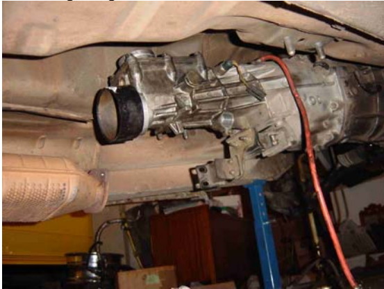
Here is my first attempt It's the one of the rb20 box with extensions welded on
