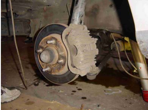
This really is a good pic to show how small the r31 standard brakes are A good move is to get the import upright that has similar sized brakes as a Silvia turbo Invite the drunken girlfriend to help and the dog Oahu so cute!
